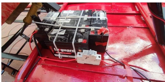
Fig 5. Battery and MCB installation
