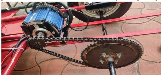
Fig 4. Mechanical connection of BLDC motor
