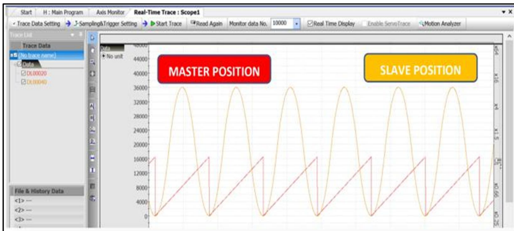
Fig. 8 Real-Time Trace of Master & slave position data
