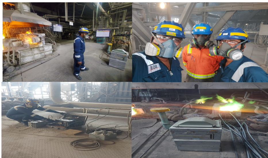
Figure – 5 Sampling Persons deputed at various emission sources for recording correct amount of emission figures in 03 shifts till 08 months viz, via Gas Analysers, SPM, SO 2 , NO x & Acid Mist Analysis – using the methodology of Iso-Kinetic & Non Iso-Kinetic Gas sampling techniques employing IS Method reference of IS:11255 & IS:5182.
