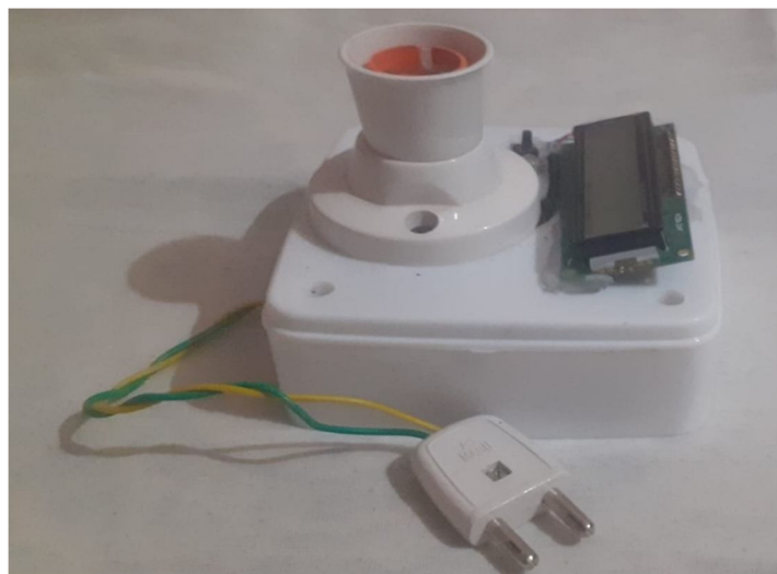
Figure 2. Prototype Kit of the Proposed EnerPulse-IoT Prepaid Smart Energy Meter
