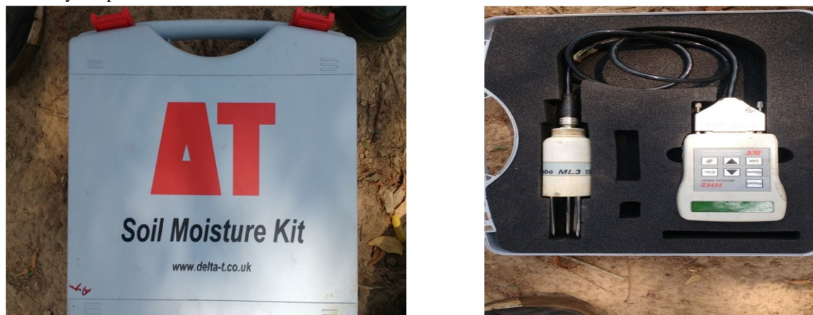
Fig.3.9 Soil moisture kit
