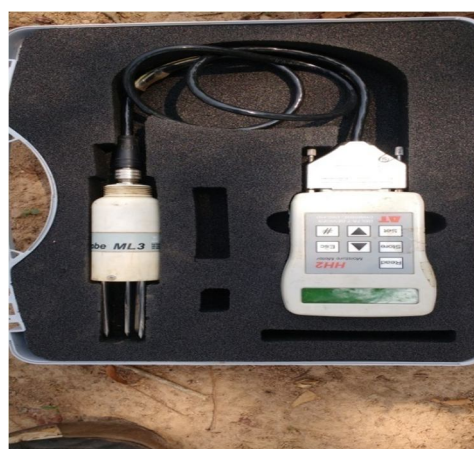
Fig.3.9 Soil moisture kit
