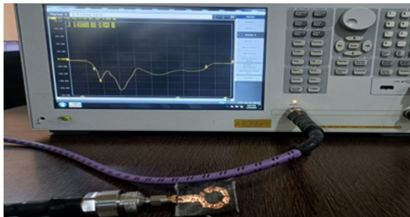
Fig 9. Proposed system hardware configuration
