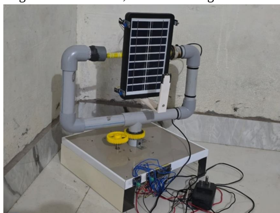
Fig. 2. Assembled dual-axis solar tracker prototype with LDR sensors mounted at the panel corners.
