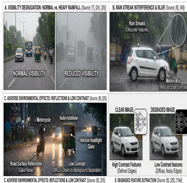
FIGURE 2. KEY VISUAL CHALLENGES FOR VEHICLE DETECTION IN INDIAN TRAFFIC UNDER HEAVY RAINFALL Demonstrates factors leading to performance decline [Source: 100], [153]
