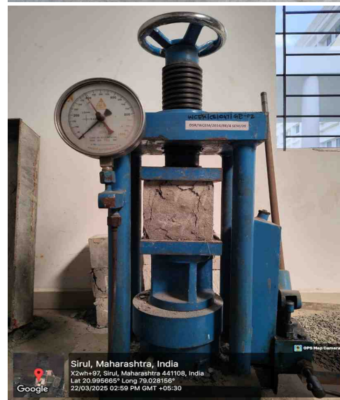
Fig. 4 Example of Cube Casting & Testing Images
