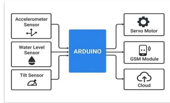
The system architecture of the proposed IoT-Based Bridge Health and Collapse Detection System is designed to provide real-time structural monitoring, early warning, and automated control using a combination of sensors, microcontroller, wireless communication, and cloud integration.
