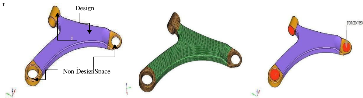
Fig.9. Optimized geometry Fig.10. Mesh model for optimization Fig.11. B. Cs for Topology optimization
