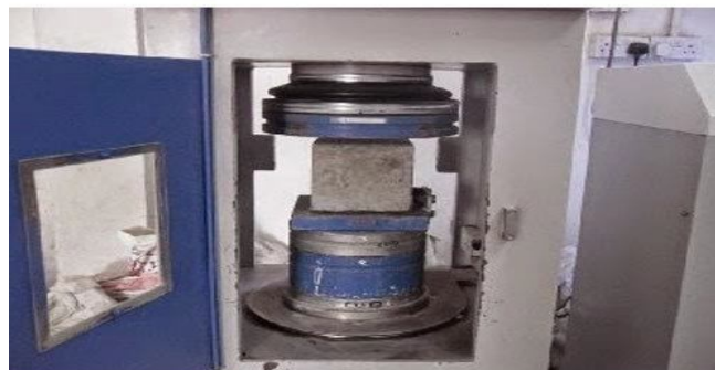
Fig. 7 Testing of cubes on Compression testing machine
