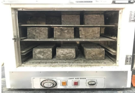
Fig. 4. Oven curing of cubes
