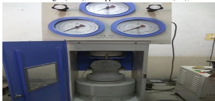
Fig. 8 Testing of cylinders on Compressive testing machine
