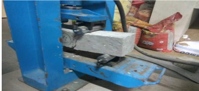
Fig. 9 Testing Beam on Flexural strength machine
