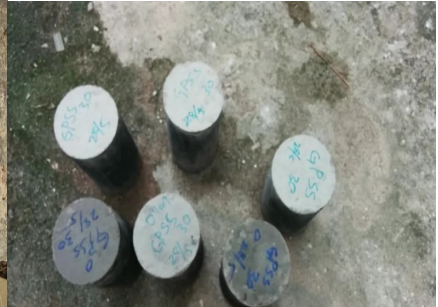
Fig. 6. Cylinders after Oven Curin
