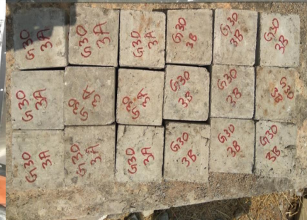
Fig. 5 Cubes after oven cured
