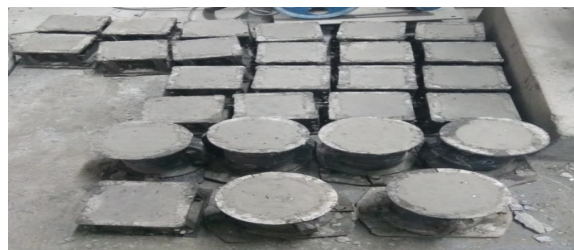
Fig. 3 Cubes and Cylinders after casted
