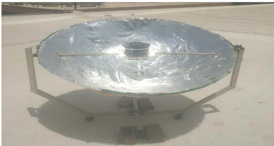
Figure 2: Solar parabolic dish collector
