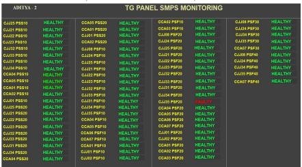
PANEL WITH ONE SMPS FAULTY IN PANEL NO.CJJ35 AND SMPS NO – PSF-20 , COLOR CODE ALSO CHANGED TO RED .
