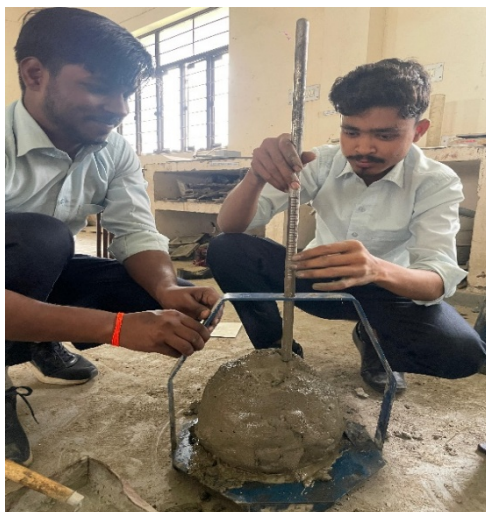
Fig.:4 Slump Test
