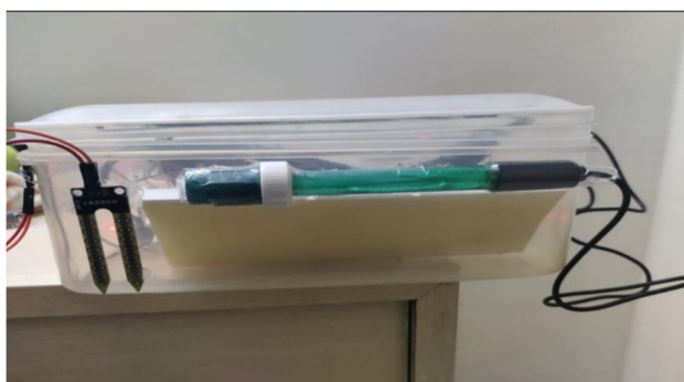
Fig 9: - Shows the mounting of PH sensor and soil moisture sensor.
