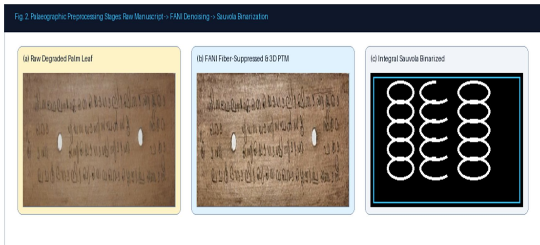
Fig. 2. Palaeographic preprocessing stages: (a) Raw degraded palm leaf, (b) FANI 2.0 fiber-suppressed surface, (c) O(1) Integral Sauvola binarization.
