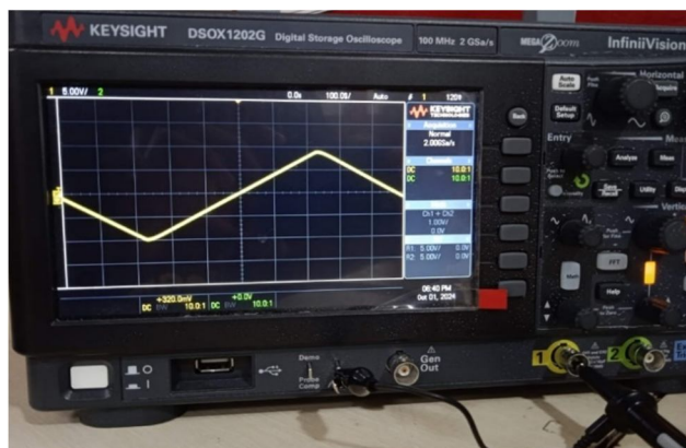
Figure 6. Keysight DSOX1202G Digital Storage Oscilloscope displaying the output – Ramp signal waveform
