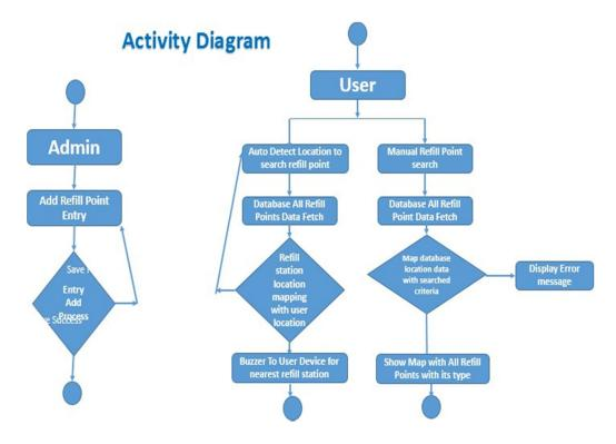
An activity diagram visually presents a series of actions or flow of control in system similar to a flowchart or a data flow diagram. Activity diagrams are often used in business process modeling. They can also describe the steps in a use case diagram.
