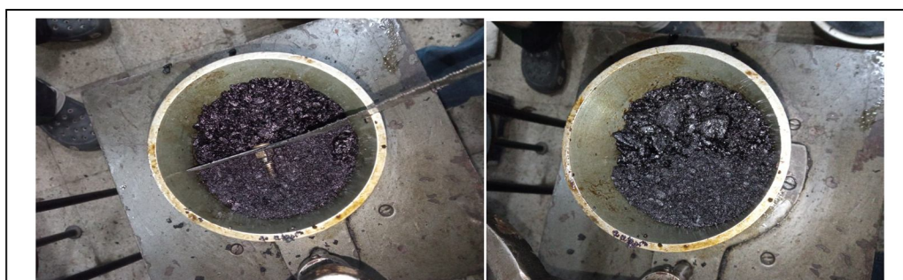
Fig 1: Preparation of composite BC-DBM Marshall specimen with glass grid reinforcement.
