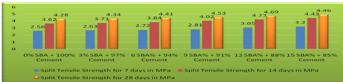
Graph 3 Development of Split Tensile strength after curing 7, 14 & 28 days for M30
