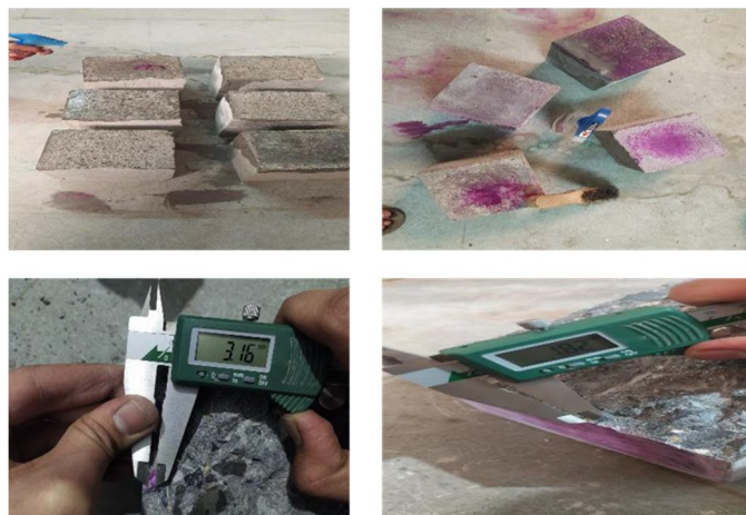
Fig. 7 Carbonation Depth Test: (As per IS-516(Part 5/Sec 3):2021
