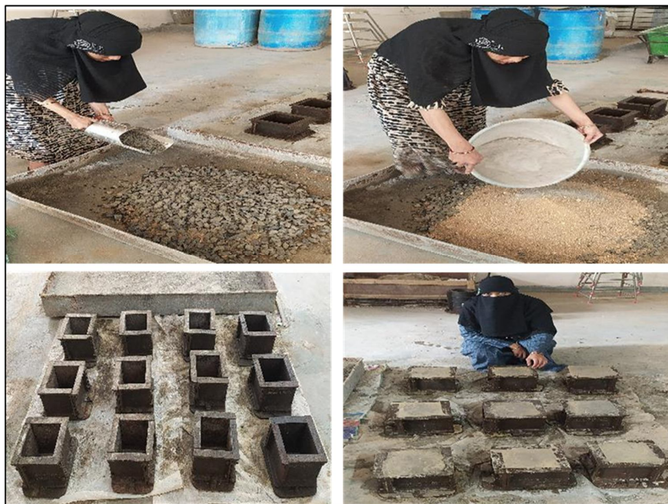
Fig. 1 Mix preparation and specimen casting
