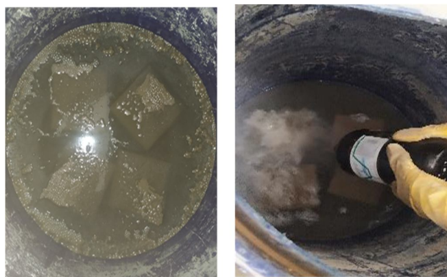
Fig. 11 Hydrochloric acid attack: As per ASTM C1898 – 20: Fig. 12 Average Comp. strength loss (%) Result after Acid attack
