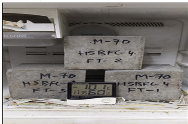
Fig. 13 Freeze–Thaw Tests of Concrete: (ASTM-C 666/C 666M – 03)
