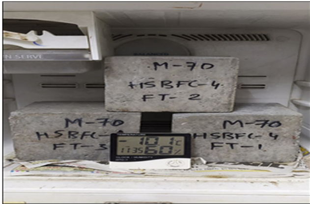
Fig. 13 Freeze–Thaw Tests of Concrete: (ASTM-C 666/C 666M – 03)
