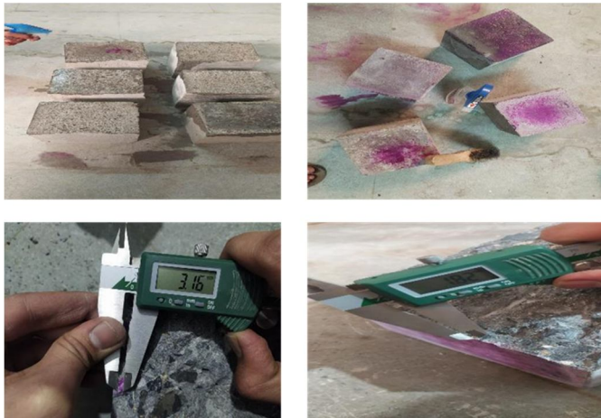
Fig. 7 Carbonation Depth Test: (As per IS-516(Part 5/Sec 3):2021
