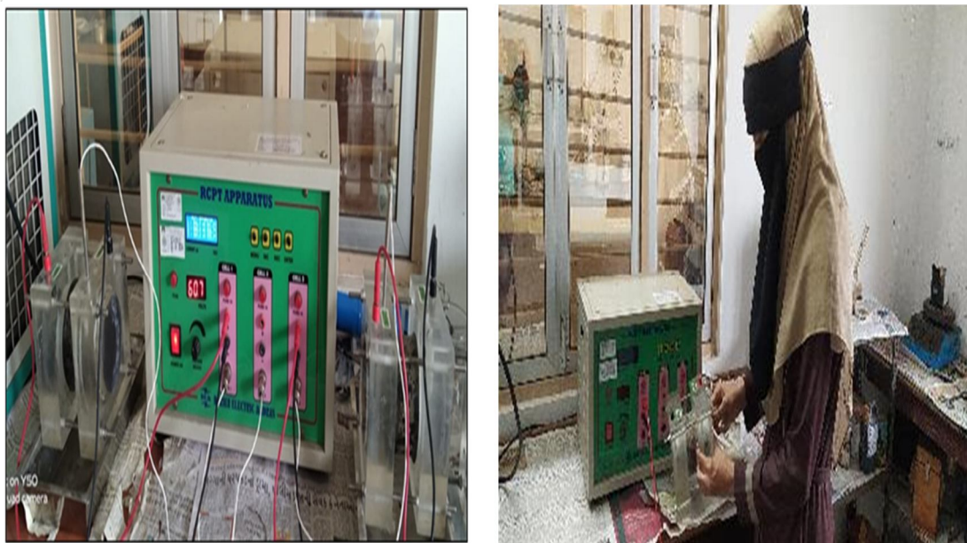
Fig. 6 Rapid Chloride Permeability Test Equipment (RCPT) as per ASTM:C1202-19
