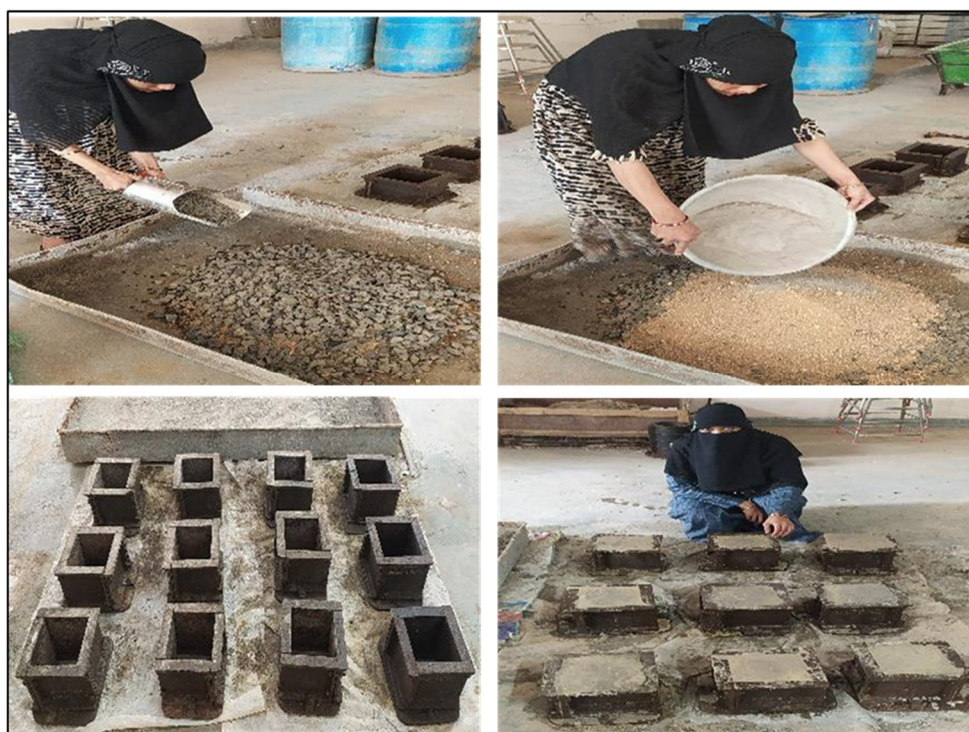
Fig. 1 Mix preparation and specimen casting
