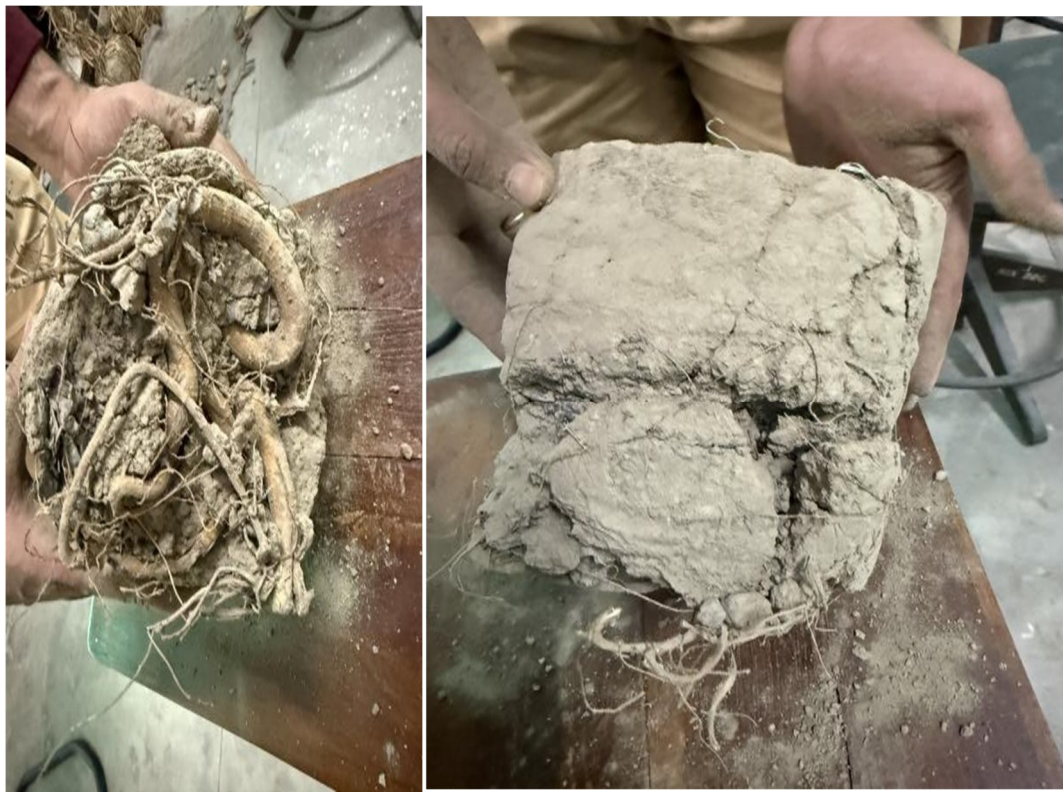
Rooted Sample After Failure
