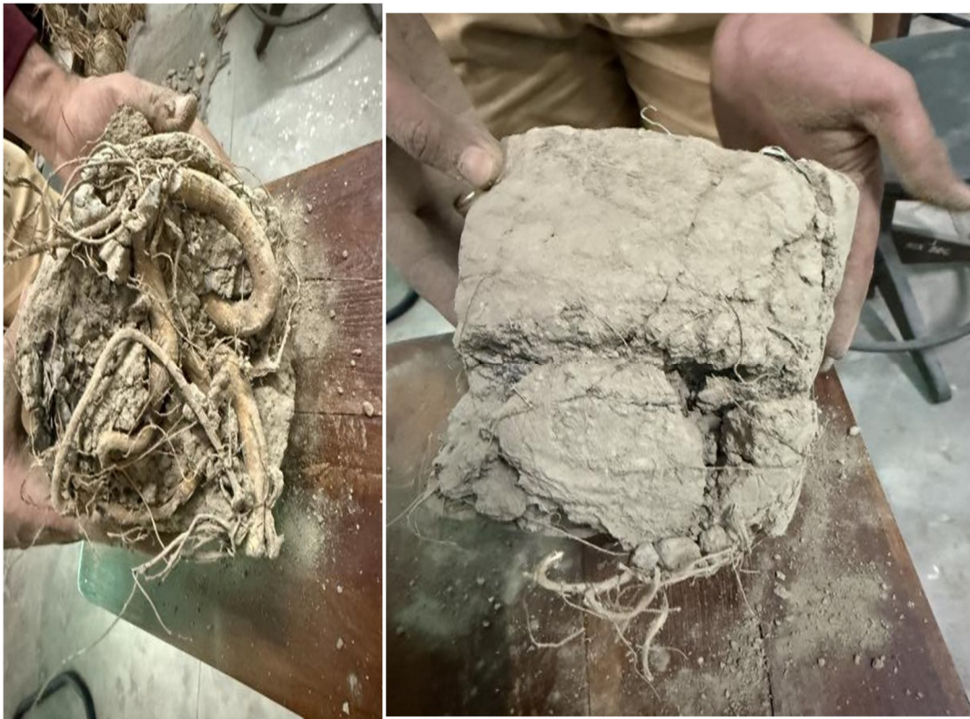
Rooted Sample After Failure
