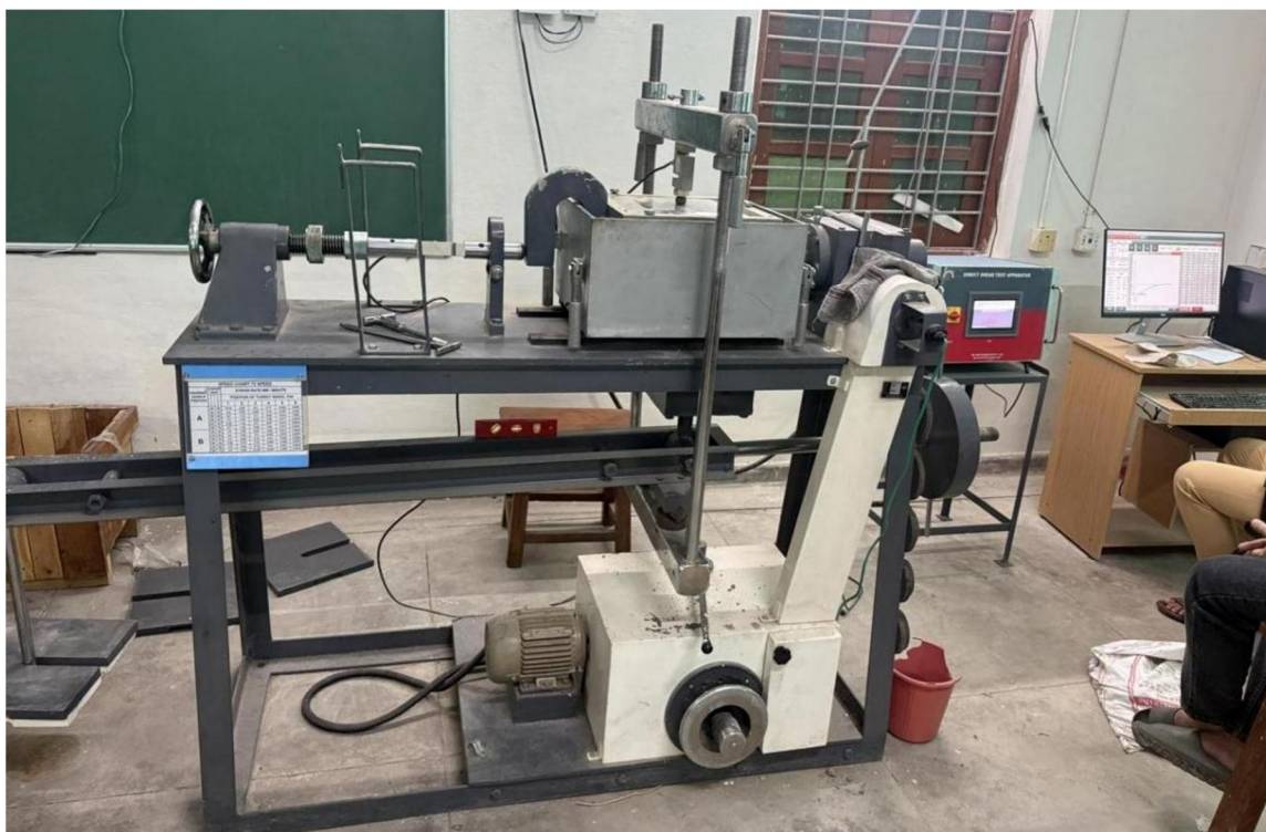
Full Setup of Direct Shear Test
