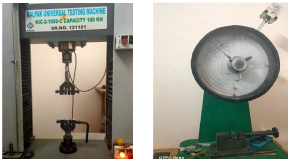
Fig 2. (a) Universal testing machine: (b) Izod testing equipment
