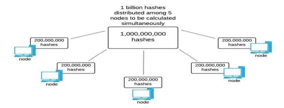
After splitting the proof of work among by the number of nodes, we can allot the range in which each device must calculate the nonce. This reduces the redundancy in computing the proof of work, and unlike the public blockchains, this is not an independent race to find the nonce, rather an organised teamwork.
