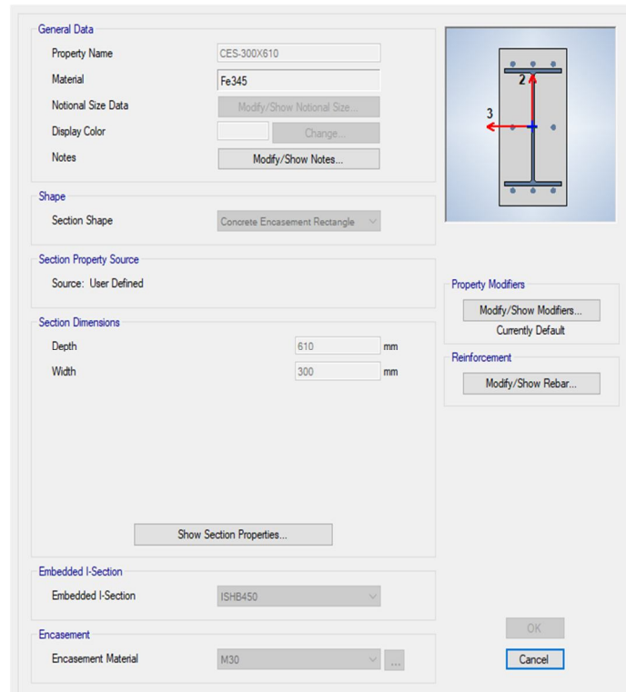
Fig. 3.6 Concrete Encased Steel Column Assigned for Modelling
