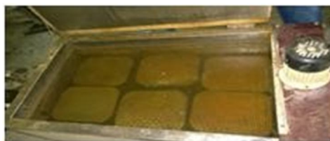
Figure 6: Accelerated Curing of Cubes in Boiler at 60°C
