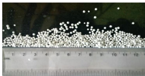
Figure 2: Size of EPS balls used in design
