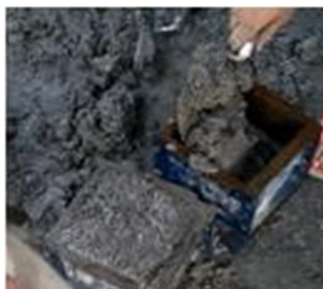
Figure 3: Filling mortar in moulds
