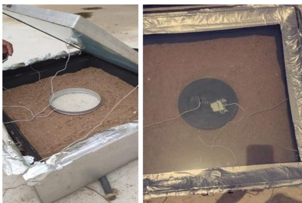
Figure 5 Solar cooker with sand as TES
