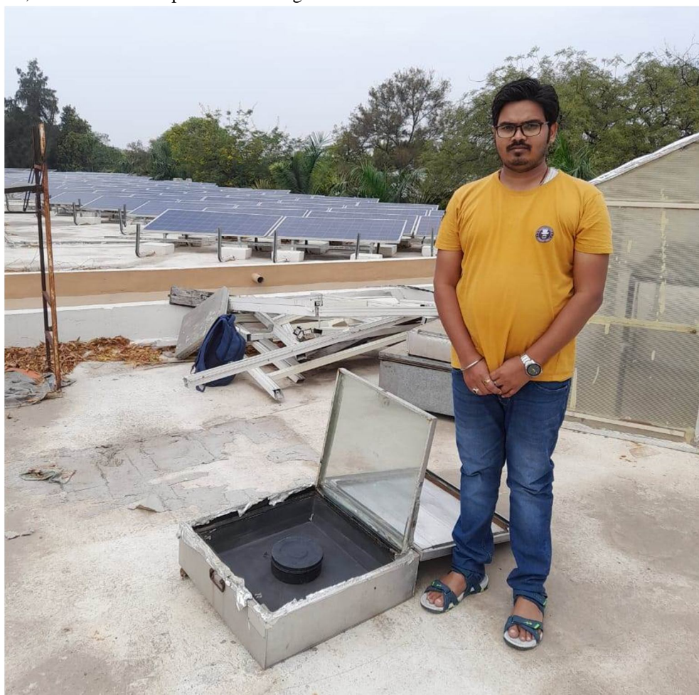
Figure 1 Solar cooker setup without TES
