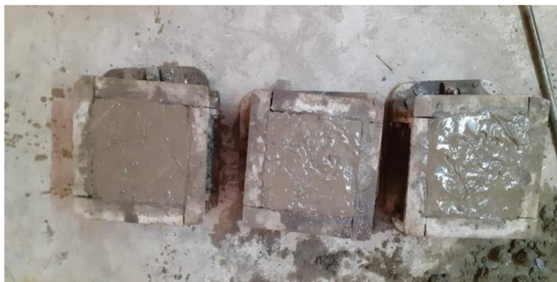
Fig 25: casting of cubes
