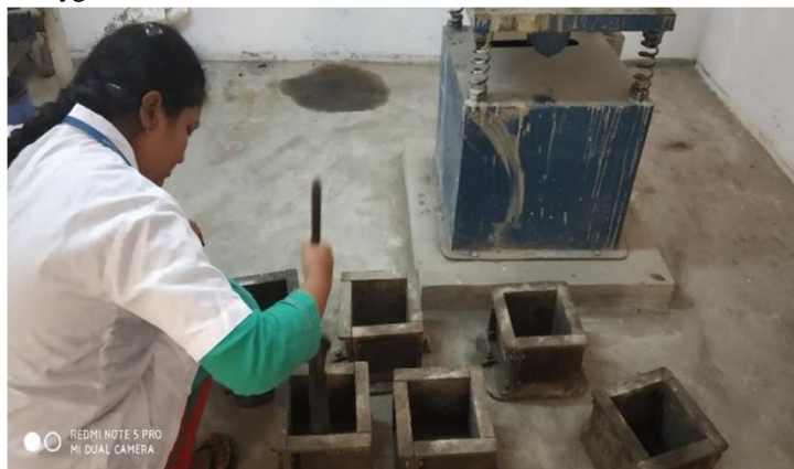
Fig 24: oiling of cubes before casting
