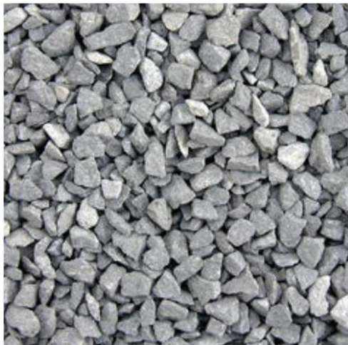
Fig 3: Crushed Coarse Aggregates
