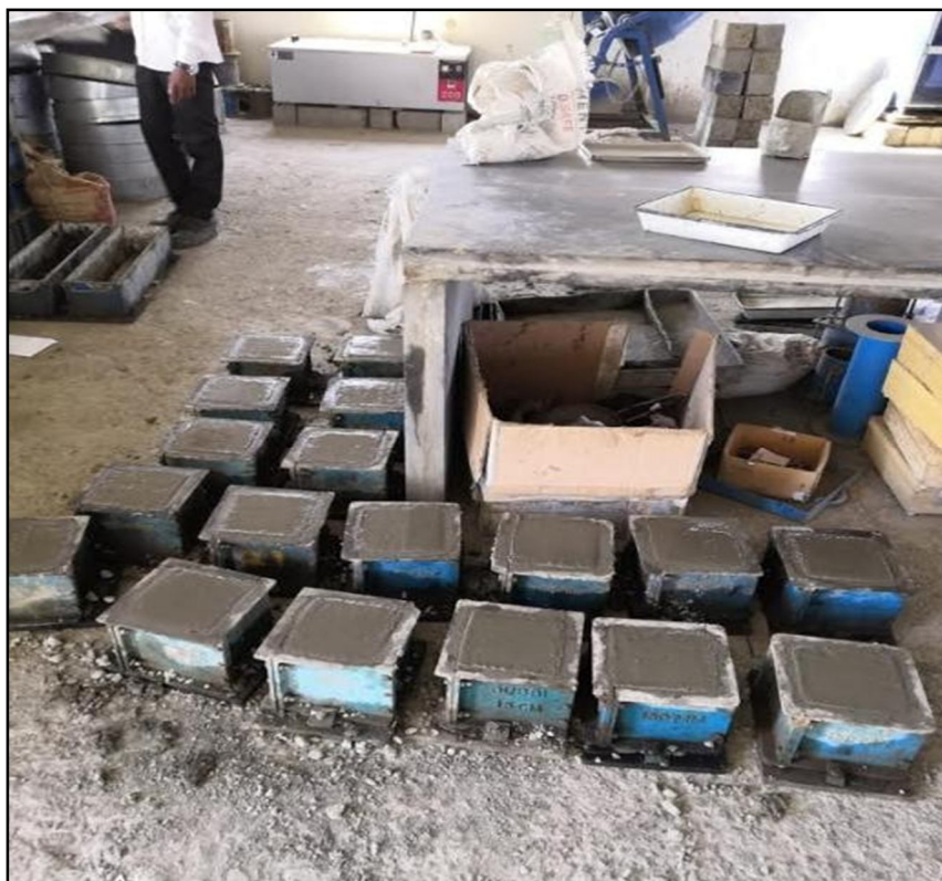
Figure 4 Casting of Cubes and Beams
