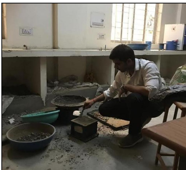
Figure 3 Sample Prepared with M-sand and Bamboo fiber
