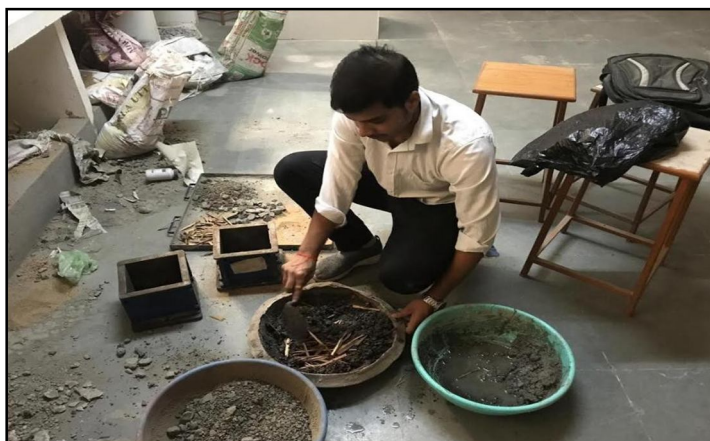
Figure 3 Sample Prepared with M-sand and Bamboo fiber
