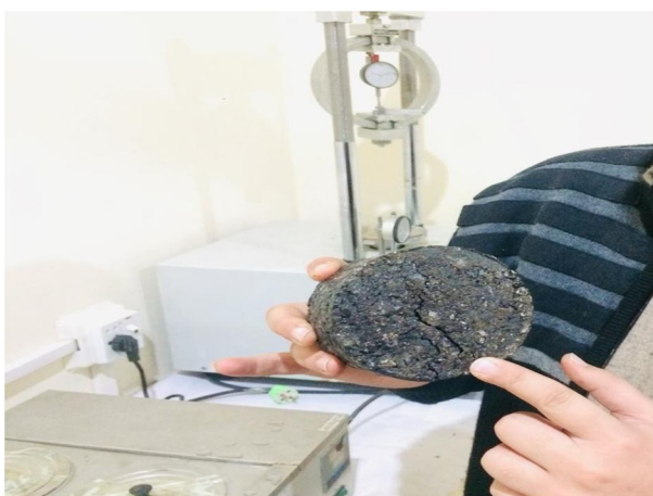
Crack after IDT testing
