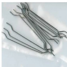
Fig.6. Steel fibers (hooked end)
