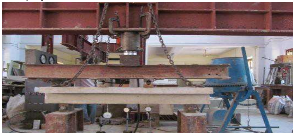
Fig 2 Experimental Setup of beam Solid beam
