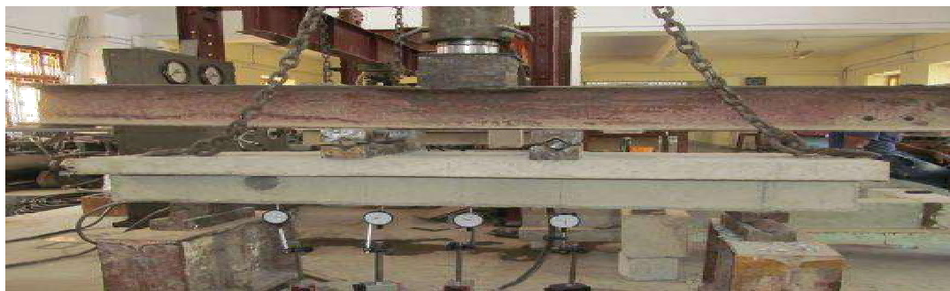
Fig 5 Experimental Setup of beam Solid beam B
