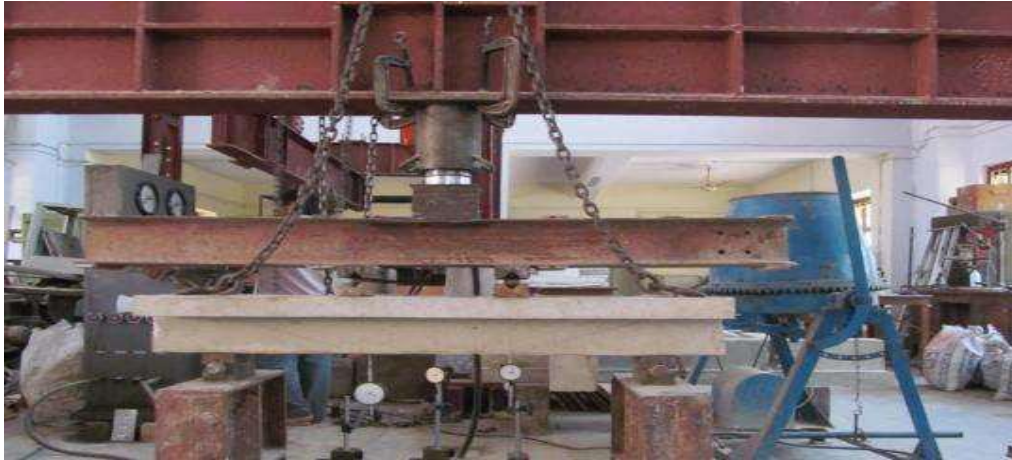
Fig 2 Experimental Setup of beam Solid beam
