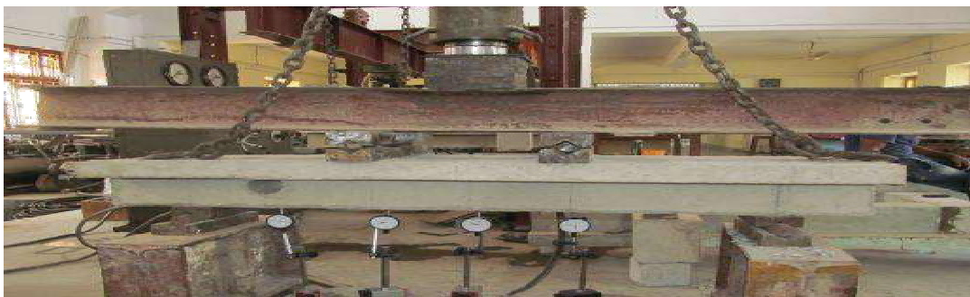
Fig 5 Experimental Setup of beam Solid beam B
