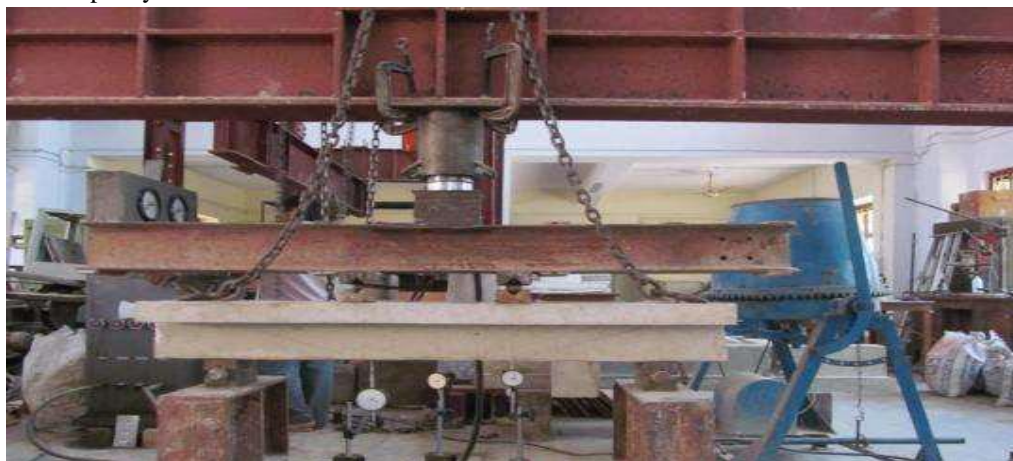
Fig 2 Experimental Setup of beam Solid beam
