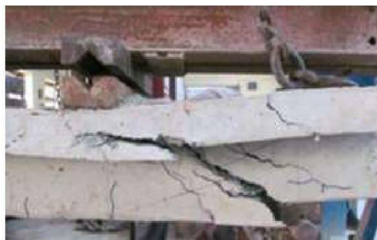
Fig 7 Widened crack at ultimate load
