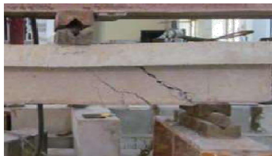
Fig 4 Widened crack at ultimate load
