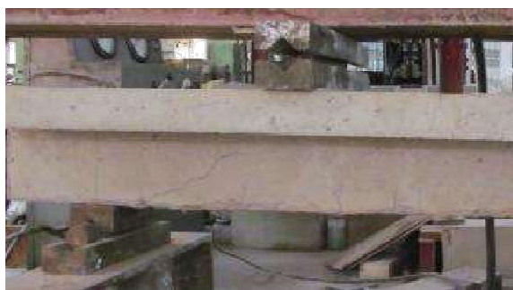
Fig 3 Hair line crack started at 110kN
