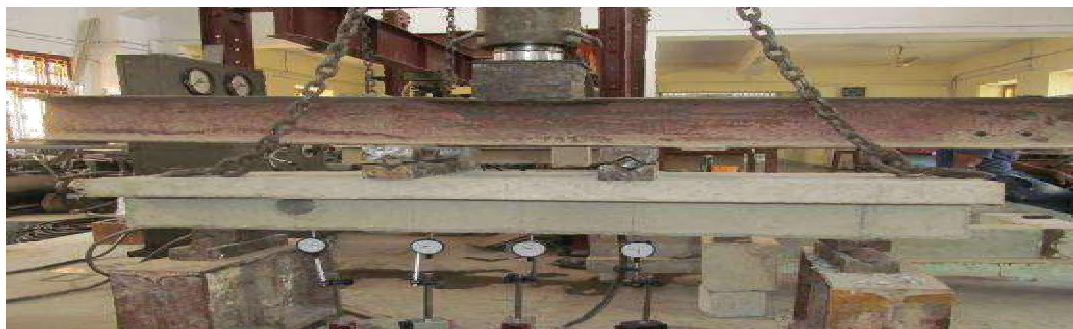
Fig 5 Experimental Setup of beam Solid beam B
