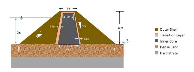
Fig.1 Geometry and materials of embankment
