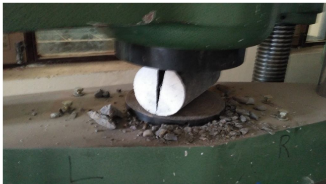
Fig. 4.9 Brittle failure of cylinder without fibre
