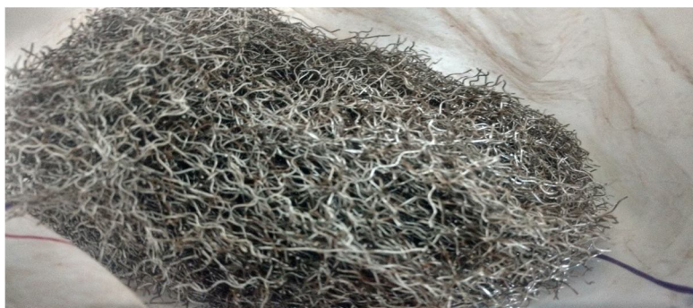
Fig. 3.2 Steel fiber used in project
