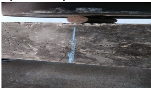
Figure 1 Experimental set up PCC beam and its crack formation
