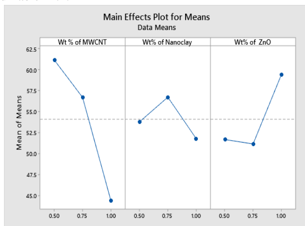
Figure 10.2 : Main Effects Plot for Means(L9-UTS)
