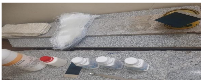
Fig 1 : Glass Fibre,Epoxy resin,Hardner and MWCNTs,Nanoclay and ZnO
