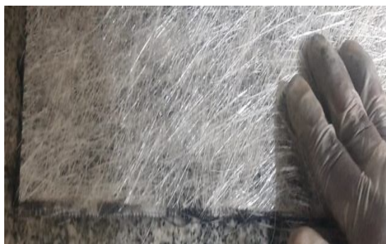
Fig 3 : Layer-02- Chopped Stranded Mat layed over layer-01
