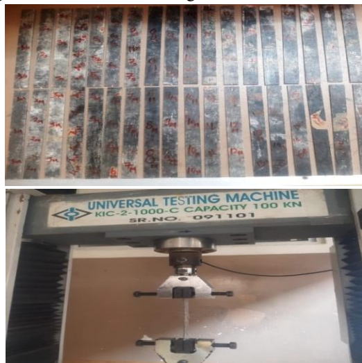
Fig 6 : Tensile test for Specimens in UTM as per ASTM Standards.
