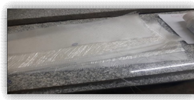
Fig 2 : 09 layers Stacking sequence arrangement of Bi-directional and chopped stranded glass fibre mat
