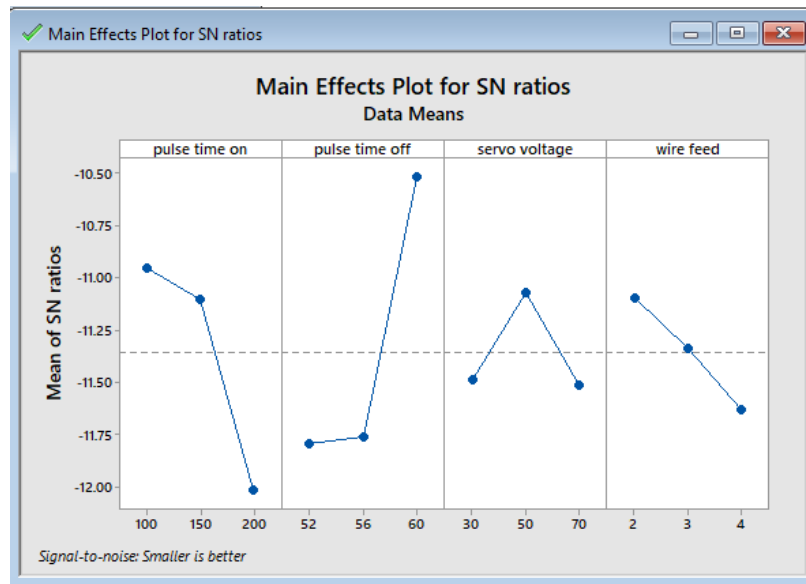
Fig12: Graph Main Effects Plot of MRR for SN Ratios
