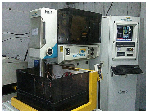
Fig2: Wire cut EDM Machine setup
