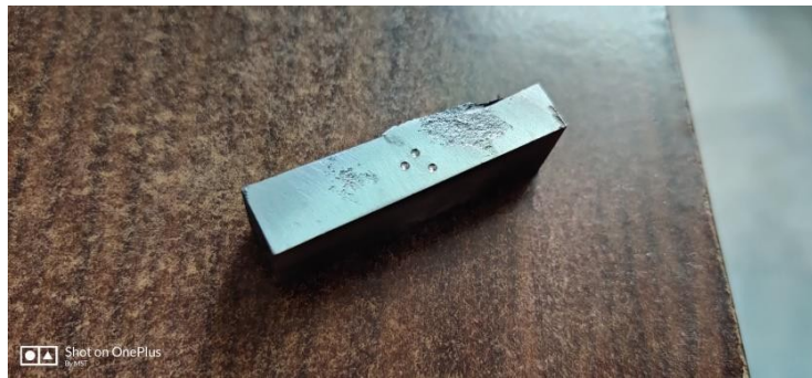
Fig8: Hardness tested work piece
