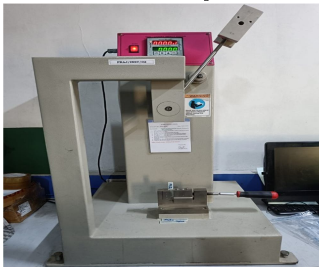
Fig : Impact testing set up of component.
