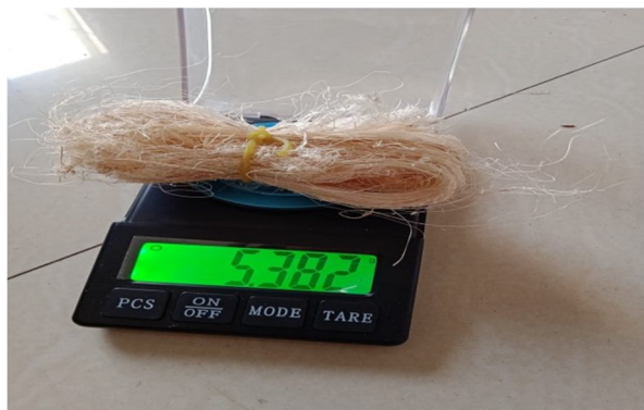
Fig. banana fiber Weight of 0.1 layer 5.382 gram used in composite making
