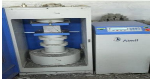
Fig.3.7 Testing of Compressive strength
