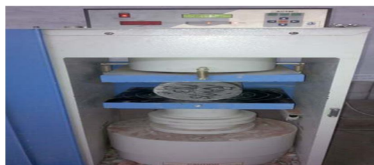
Figure 3.10: Splitting Tensile Strength
