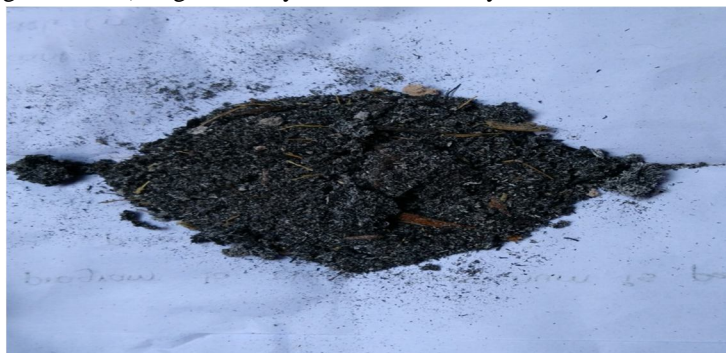
Fig -5: 70% of particle passing 0.090mm fine Bagasse ash particles
