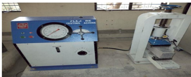
Fig.3.9 Testing of Flexural strength
