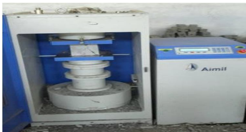
Fig.3.7 Testing of Compressive strength
