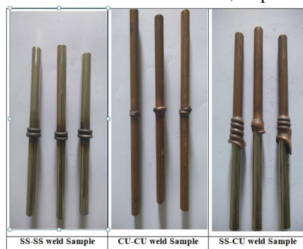
Fig 2 Friction welded dissimilar welded specimens
