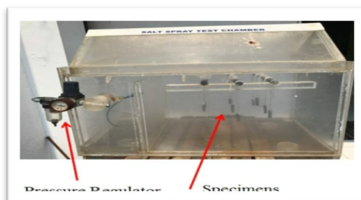
Fig 12 Salt spray corrosion setup
