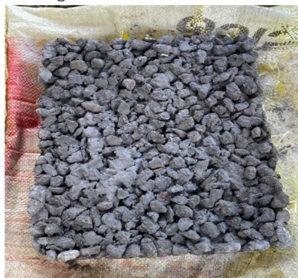
Figure: pervious concrete sample showing its coarse aggregate structure
