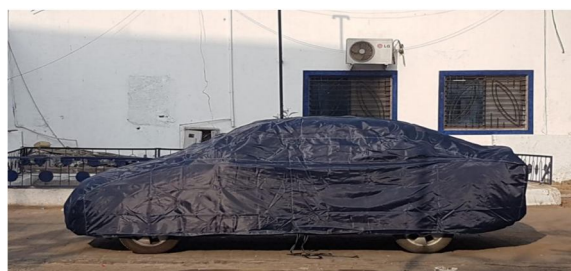
Fig 5 Sedan vehicle covered with heat-resistant roof-top taffeta material
