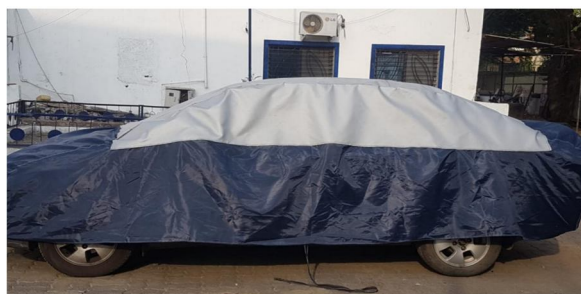
Fig 6 Sedan vehicle covered with heat-resistant roof-top double-sided silicone-coated fibreglass cloth
