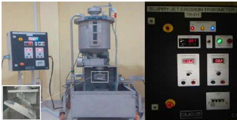
Fig.1. Slurry jet erosion testing machine
