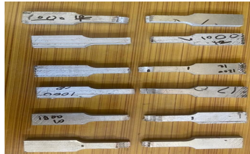
Fig 2– Work specimens after tensile test on UTM
