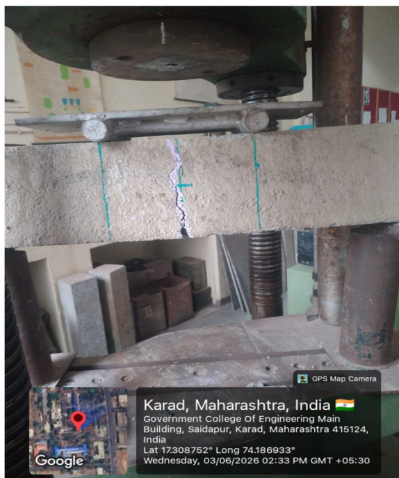
Fig. 3: Beam flexural strength testing
