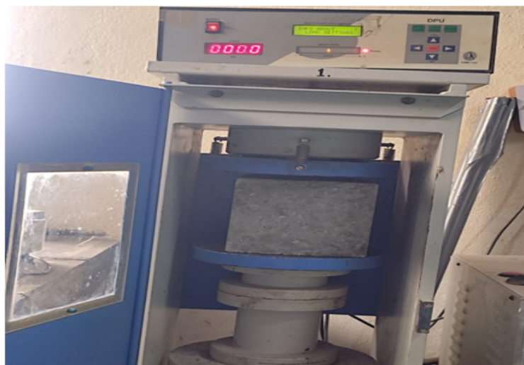
Compression Strength Test Result on normal concrete
