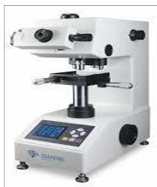
Figure 7: Vickers Hardness Test Equipment
