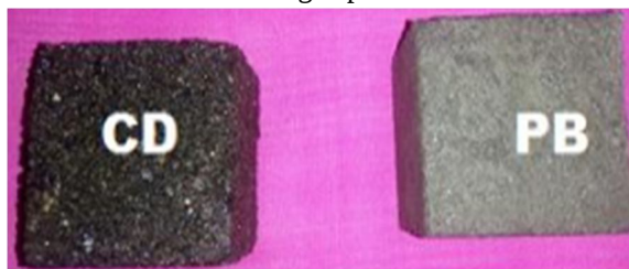
Fig. 1. Appearance of sand-plastic specimens prepared from waste compact discs (CD) and plastic bottles (PB).
