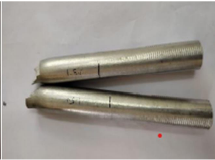
Figure 8: Tensile tested Al6061 + 1.5% ZrO 2 specimen
