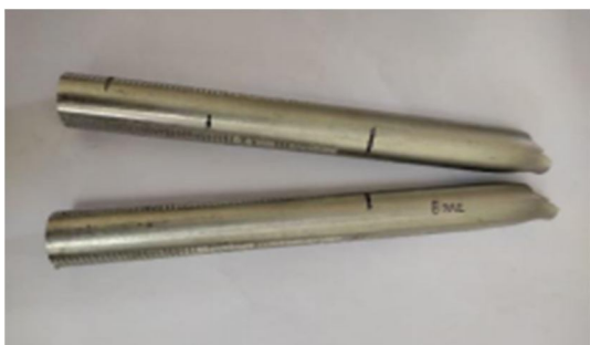
Figure 5: Tensile tested Al6061 specimen
