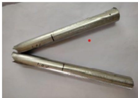
Figure 7: Tensile tested Al6061 + 1.0% ZrO 2 specimen
