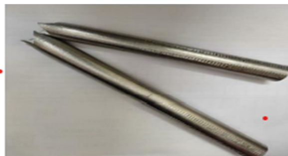
Figure 6: Tensile tested Al6061 + 0.5% ZrO 2 specimen
