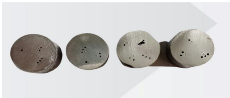
Figure 14: Hardness Tested Specimen
