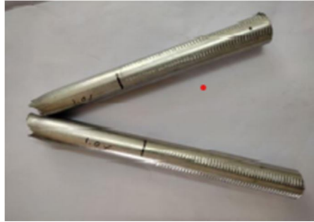
Figure 7: Tensile tested Al6061 + 1.0% ZrO 2 specimen
