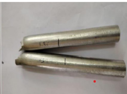
Figure 8: Tensile tested Al6061 + 1.5% ZrO 2 specimen
