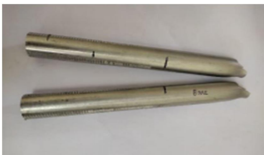
Figure 5: Tensile tested Al6061 specimen
