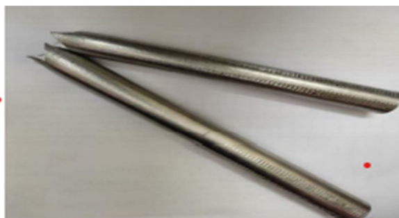
Figure 6: Tensile tested Al6061 + 0.5% ZrO 2 specimen
